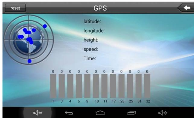
With this application, you can check the status of the GPS receiver without any navigation software.
